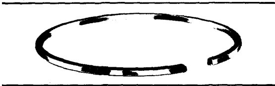
Figure 5-6. "H" Type or Single-Piece, Non-Ventilated Beveled-Scaper Style Oil Control Wiper Ring
