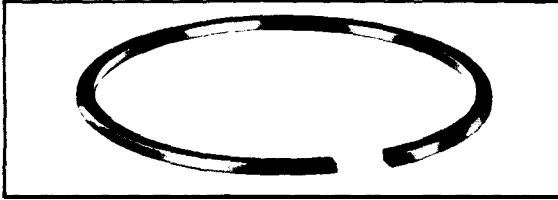
Figure 5-5. "B" Type or Single-Piece, Taper-Faced Style Compression Ring
